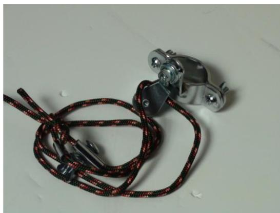
The purpose of this part is to provide resistance at the toe or front of the foot. Some riders tend to point their toes downward. This is designed to provide resistance against that tendency and help keep the foot in a level riding position.
