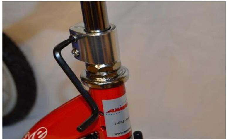
**⚠ CAUTION: HANDLEBAR STEM MUST BE INSERTED INTO FORK HEAD TUBE TO AT LEAST MINIMUM INSERTION LINE (HASH MARKS). WHEN INSTALLED PROPERLY HASH MARKS ARE NOT VISIBLE.**
