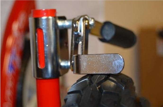
**NOTE:** Top of the loading brake should be flush with the top of tube. Make sure that the lever is not touching the tire. The handle needs to be in line with the tire and point toward the front of the tryke.
