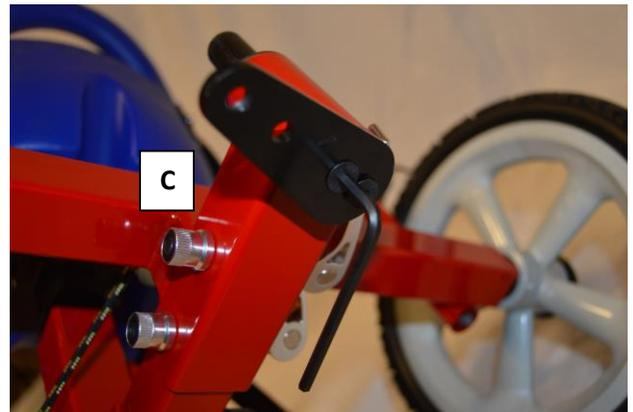
Recommendation: Add Loctite to screws before installation.
