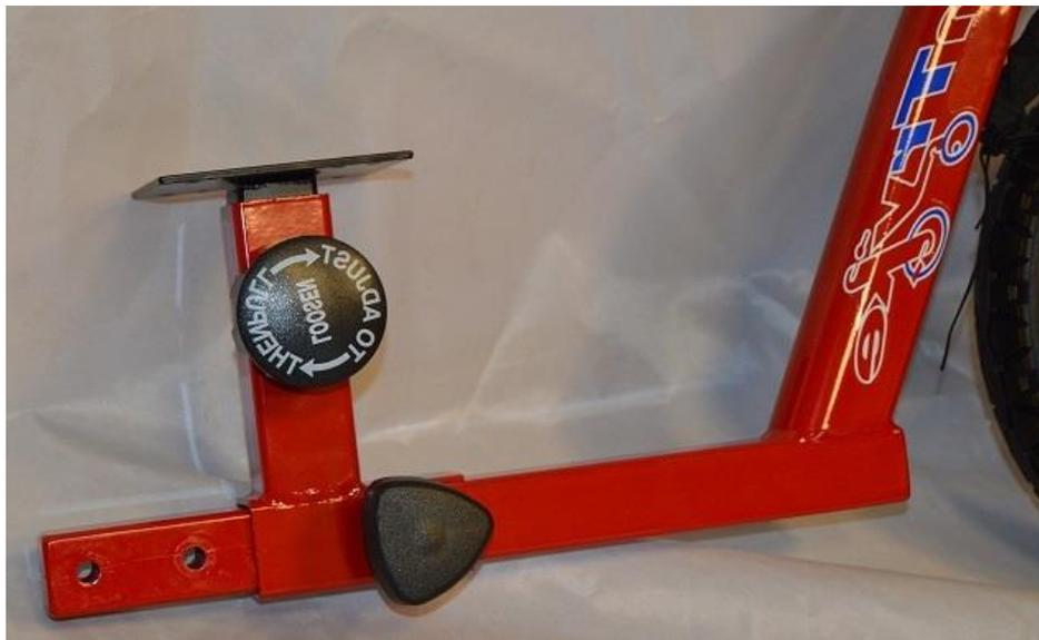
**NOTE:** The two seat post bracket knob holes should be on the bottom right side of the tryke.
