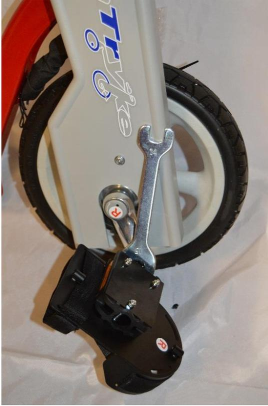
**TIP:** Pedals and pedal cranks are labeled “R” (right) and “L” (left).
