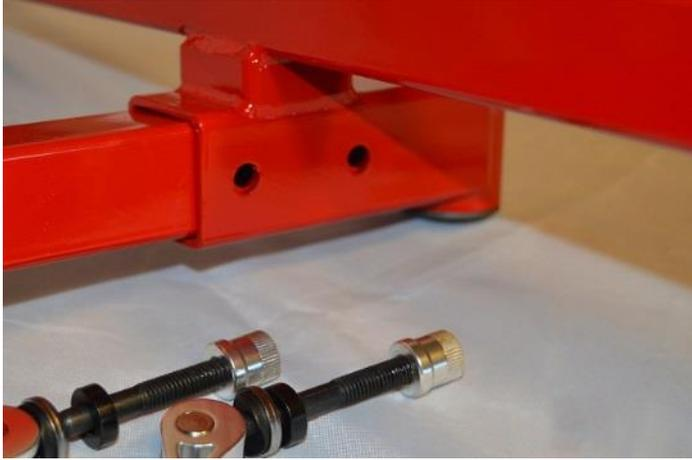
**NOTE:** Pay attention to orientation. Rear axle is on top of the frame assembly and vertical post for loading lock is on right side of tryke.
