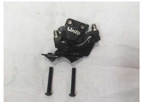
6. Insure brake pads slide smoothly over brake disk.
