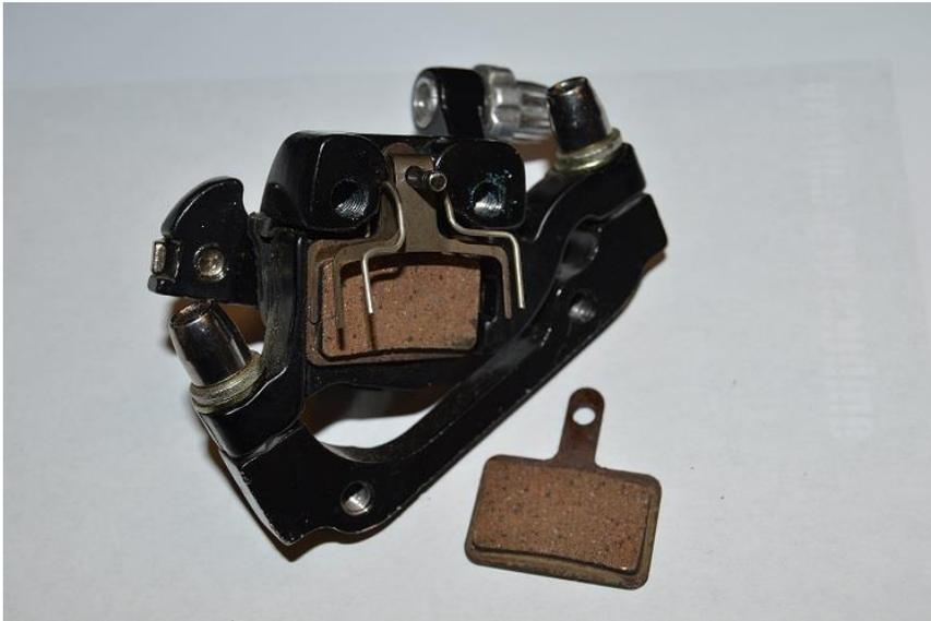
**Step 5:** Reinstall new brake shoe pads to match the preexisting setup. Replace back cover using the 5mm Allen/Hex wrench.
