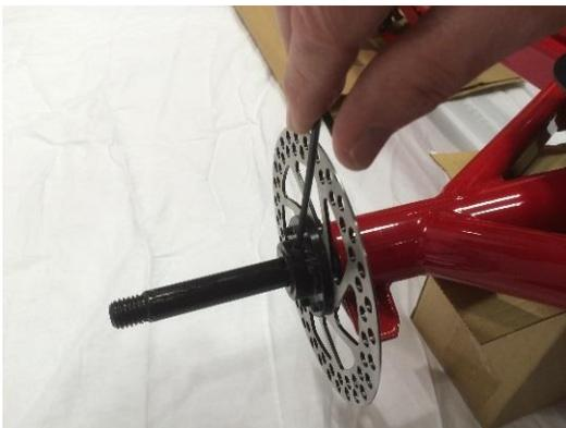
3. Install rear wheels (do not use the 22mm silver spacer tube on the left side axle when you are installing the rear steering kit).
