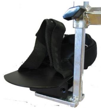
10) To mount the foot platform on the AmTryke, unscrew the securing collar adjustment knob and remove the washer and bolt. Place the collar over the frame and re-install the securing collar washer, bolt and adjustment knob. Tighten the knob until the foot stabilizer does not slide or move.
