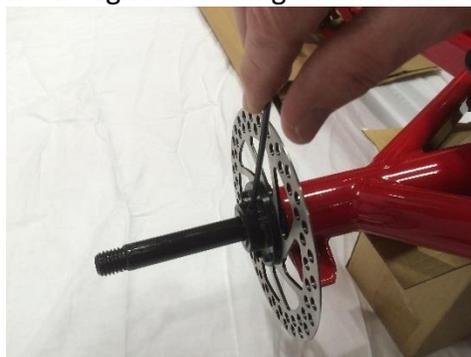
3. Install rear wheels (do not use the 22mm silver spacer tube on the left side axle if you are installing the rear steering kit).
