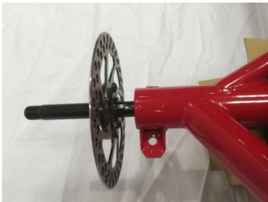
2. Install the 3mm set screw through rotor using a 3mm Allen wrench, tighten securely.
