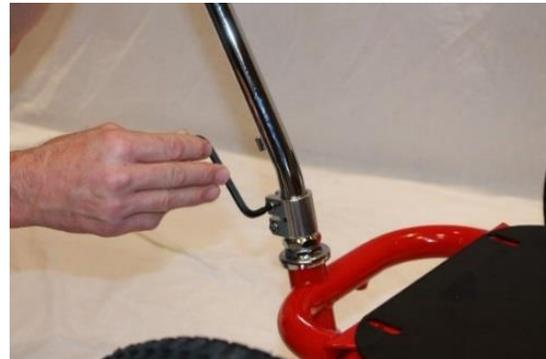
Once the steering bar is fully inserted—align with front wheel for straight ahead position—then tighten the two 5mm Allen screws on the cinch collar.
