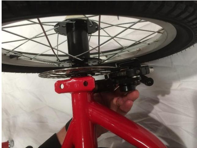
c.) Put in black bolts with 5mm Allen wrench. Hint: tighten the rear bolt first as it will touch the bracket. Then tighten the front bolt until the brake is secure. Be sure both sides of the brake bracket contacts the red rear axle tube evenly.
