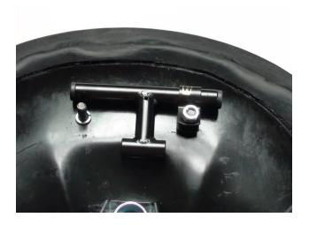
5) Slide the clamp that you removed over the other long end of the H-bracket, place clamp over threaded stud of tractor seat, re-install the nut by turning clockwise.
