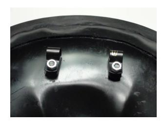
3) Remove one of the nuts that secure the clamp onto the bottom of the seat and remove the clamp.
