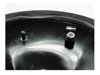
4) Slide one of the long ends of the H-bracket onto the clamp on the bottom of the seat.
